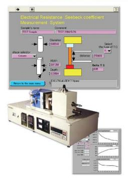
It's easy to accurately measure the thermoelectric effect with the ZEM-3 from ULVAC. ZEM-3 automatically measures both the Seebeck Coefficient and Electrical Resistivity of bulk samples, thin sheet or deposited thin film thermoelectric materials.
